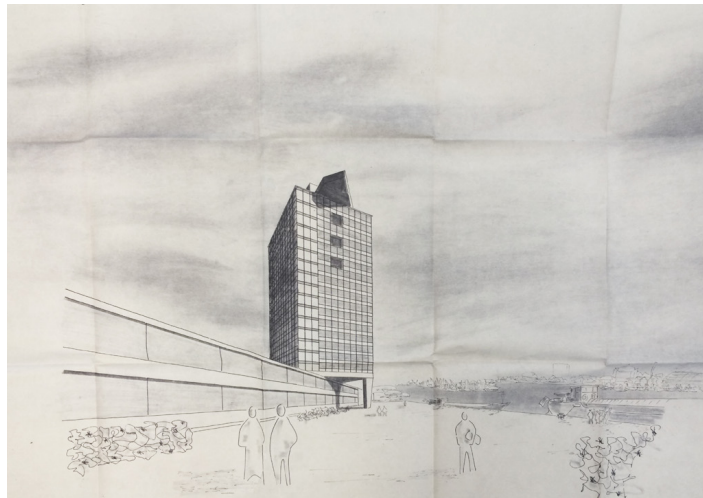
Preliminary sketch with the tower turned 45° above a low-rise volume. Image: Sandra Guarda, "The Importance of Being Overhoeks"
